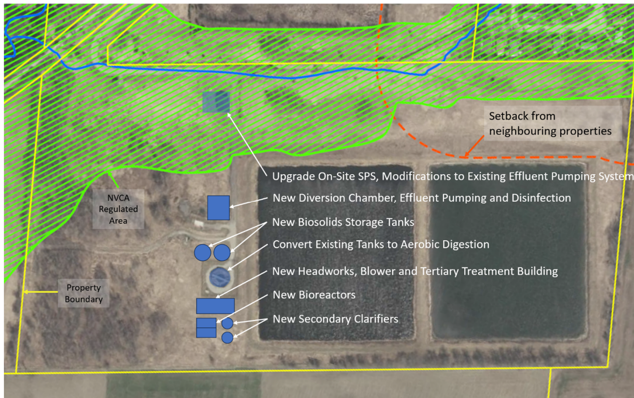
Conceptual Layout for Option 1 – Extended Aeration with Tertiary Filtration
